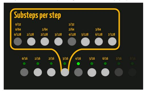
The sub steps define a step pattern that is played when the corresponding main step is active. The Sub steps can be used to create flam/roll sounds on a particular step, or to play a note between the 16<sup>th</sup> notes represented by the main steps.
